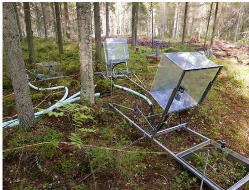
Figure 4. In 2019, six automated chambers for forest floor greenhouse gas flux measurements were made operational at Ränskälänkorpi site. Photo: Tuomas Laurila.
